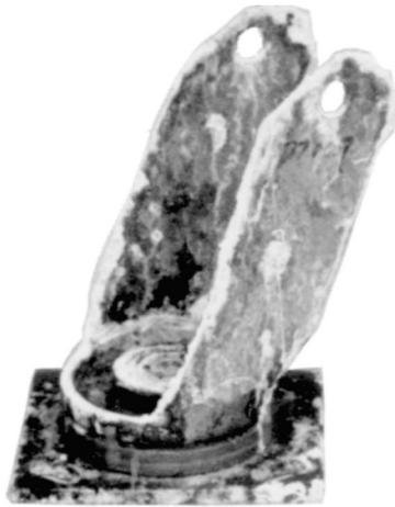
Dichromate Zinc Plating failed after 72 hours.
